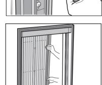
② Adjust the inclination of the Side Bar so it is straight.
