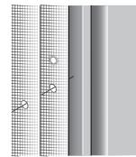
A5 Due to the product's configuration, the pleated net cannot be replaced by itself. The entire Screen Door Unit needs to be replaced. Consult your dealer for best alternatives. Small holes may be covered with commercially available patches.
