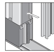
4.Re-attach the Magnet Holder Re-attach the Magnet Holder to the Slide Bar when the adjustment is complete.
