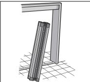
2 Tilt the Screen Door Unit and remove from the Top Rail.
