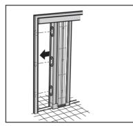
5 Slide the Screen Door Unit towards the door installation frame keeping the bottom of in contact with the Bottom Rail. Press firmly to attach in place.
