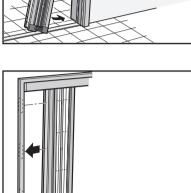
4 Check the Screen Door Unit does not come off of rail and press firmly towards the door installation frame making sure the Anchor Plates fasten in place with an audible "click".
