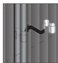
Install Link Spring The Link Springs are attached when delivered. In case they are off-position, re-attach at equal points.
