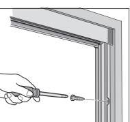
7.Installation of stop post with magnet
