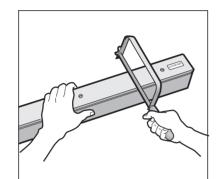
Even though the product is made to measure, if the install location is still narrower than the product, cut the Top Rail and Bottom Rail to match installation width. 3. Cut the Top Rail
