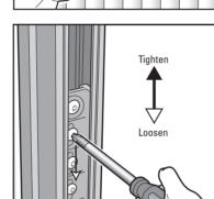
3 Loosen the screw on the Wire End Tail (Yellow), Refer to
