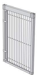
(2)Loosen the wire adjustment screw on Stile post and move it towards the direction where the wire tension gets tighter and fix it with screw.
