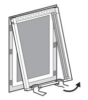
(6) Take away the screen unit for the next procedure Hold the Bottom rail ( or Stile post, Stop post ) with hands and pull it. Then the screen unit will be taken away from the frames.
