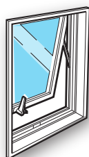
横滑り出し窓 Top-hinged outswinging window
