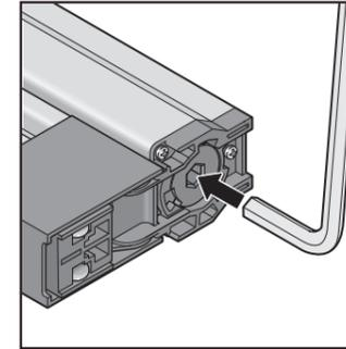
If the screen unit is not retracted into the roller case when it is closed, insert the tip of the hexagonal wrench into the hole at the bottom of the roller case cap in the roller case, lift it up a little bit and rotate it two turns in the direction of the arrow indicated to the left.
