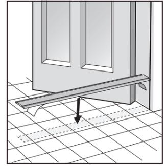
Peel the white double-sided sticker off the bottom rail and place it in line with the marked position and push the bottom rail strongly down along the floor so that it reaches the side of Stile post. Note that there is some space on the side of Stop post.
