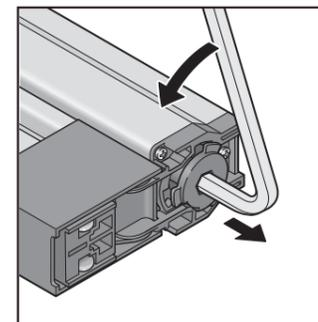
When the screen unit is retracted into the roller case with high speed right after you open it, insert the tip of hexagonal wrench into the hole at the bottom of the roller case cap in the roller case, lift it up a little bit and rotate it two turns in the opposite direction of the arrow indicated to the left. And put back the roller case cap into the roller case keeping it as it is.
