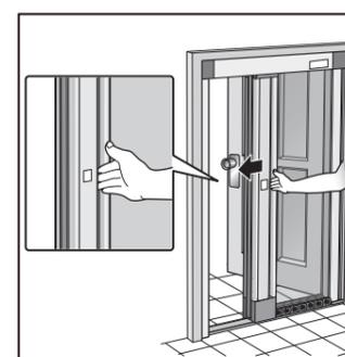
Hold the center of the sliding bar for open and close operation. A magnet is installed inside the stop post to keep the screen unit tightly closed.
