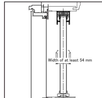
Choose an installation location at which the screen door can be opened and closed unimpeded.
