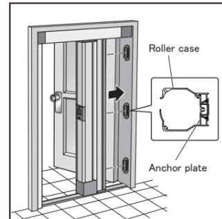
① Draw a line along the frame on the side of stile post from top rail down to bottom rail.
