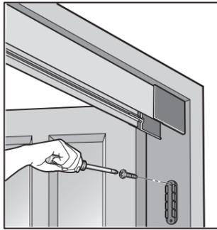
② Temporarily place the anchor plate in the position marked after peeling the tape off the anchor plate. Fix it with the tapping screws.
