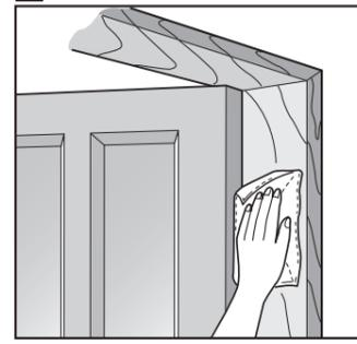
Wipe away all oil residue, dust, water, sand and mud from the installation surface and the floor and then wipe these surfaces with a dry cloth to ensure that the product is installed properly.
