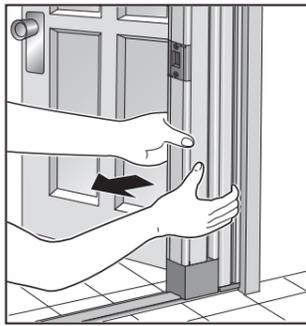
① Place your hands on the stile post as shown in left drawing. Pull it hard so the unit is pulled off and only anchor plate remains on the wall. Pull it from the bottom end so the anchor plate can be detached easily. Pay close attention and make sure that the unit will not lose its balance falling to the ground.
