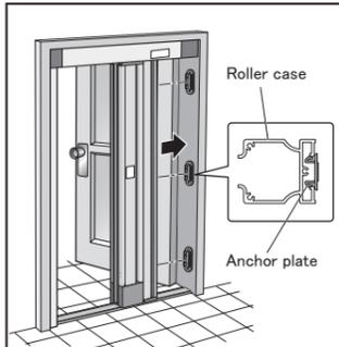
Follow the same procedure as that of anchor plate and push it on to the anchor plates so that it clicks on it firmly.
