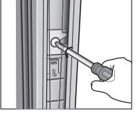
② Adjust the inclination of the sliding bar so it is straight.
