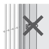
A6-A7 The screen door works by housing the scorpion tail inside the sliding bar and stile post. Therefore, you should never attempt to drill holes in the (aluminum) material and screw on a handle or lock. If you have attempted to do this and the screen door does not move even when the screws are removed, or if the material is dented, you must replace the entire screen door unit. Please consult your dealer.
