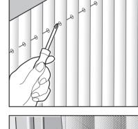
③ The screw to adjust the wire is attached around the bottom of the Slide bar.
