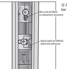
4 Check the positions of the screw which adjusts the sliding bar inclination and the screw which adjusts the wire tension.
