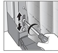
$\mathbb{Q}2$  There are small pebbles, sand, dust and mud on and around the rails, preventing the screen door from moving smoothly.
