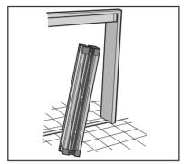
② Tilt the screen door unit and remove it from the top rail.
