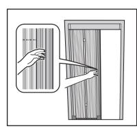
Hold the groove around the center of the Slide bar and make the open & close operation.
