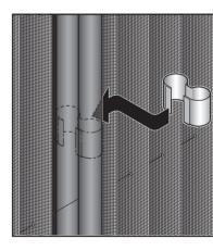
11.Install Link Spring The Link Springs are attached when delivered. In case they are off-position, re-attach at equal points.
