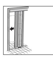
④ While making sure that the bottom of the screen door unit does not stick up from the bottom rail, align the stile post with the projections on the anchor plates and press in until you hear the click that indicates that the screen door unit is fastened in place.
