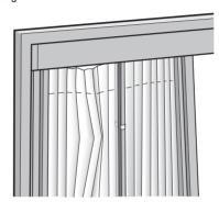
A3-A4 While making sure the screen door does not fall, return the scorpion tail to its proper position at the top of the pleated net.
